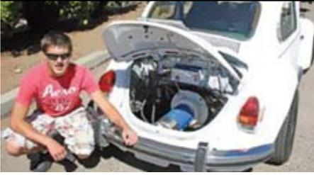
U.S. high school student Stark Ashton recently transformed his grandfather's 1972 VW Beetle into an electric vehicle. The cost? around \$4,000. He equipped the Beetle with nine golf cart batteries, used to power a single motorized shaft which can propel the car for nearly 80km on less than 10 cents worth of electricity. The converted Beetle is able to reach speeds of 72 km/hour.
